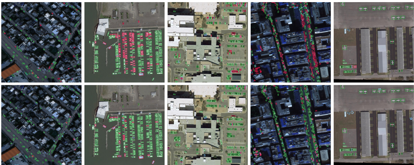
Fig. 7. Visualization analysis of the predicted results. The first row shows the predicted results by the Oriented R-CNN while the second row shows results from DCFL on the AI-TOD-R dataset. True positive, false negative, and false positive predictions are marked in green, red, and blue, respectively.
