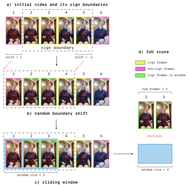
Figure 1. The process of receiving IoU scores. (a) Consider the initial video, where the sign is between frames 2 and 5. (b) Random shift the sign’s boundaries by one frame to enhance model robustness (see Section 3.1 for details). (c) Collect frames by sliding a window of size 3 across the video. (d) Calculate IoU scores by dividing the number of sign frames in the window by the window size and adjust the classification scores (see Equation 2).
