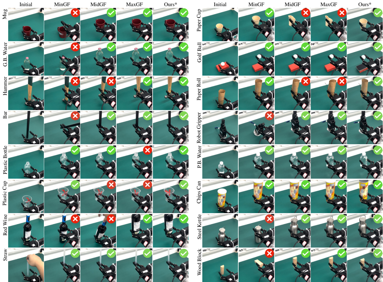
Figure 10. Complete robot grasping experiment results. The 16 test cases along with results in robot grasping experiments are listed. We compare our proposed method (right) against three baselines (middle columns), starting from initial configurations (left). You can view the MP4 videos of the experiments in our project page.
