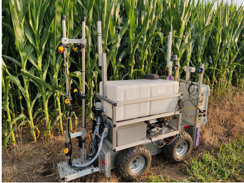
Figure 2: The under-the-canopy robot equipped with Jetson Orin and Luxonis OAK-D Pro for image acquisition.
