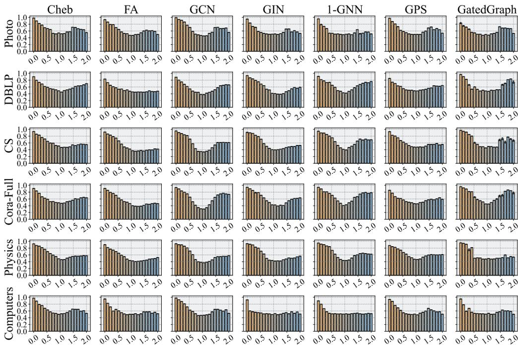
Figure 13: The accuracy curves of different GNNs (Cheb, FA, GCN, GIN, 1-GNN, GPS and GatedGraph) in the whole spectral domain. In each subplot, the  $x$ -axis represents the frequency and the  $y$ -axis represents the accuracy of GNNs in the node classification task with the ground truth labels derived from the associated frequency bin.
