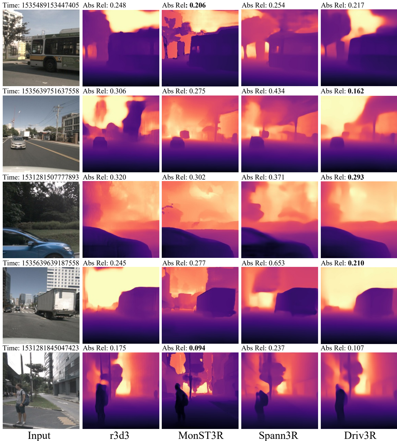
Figure 6. Additional Visualization Results of Depth Prediction on nuScenes [4] dataset. While MonST3R [52] demonstrates more refined depth prediction in certain scenarios, Driv3R delivers comparable performance with a 15x faster inference speed, outperforming methods which rely on global alignment optimization to reconstruct large-scale dynamic scenes.
