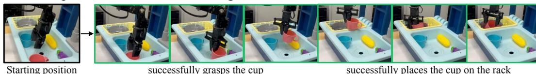
**Figure 4:** Evolution of learned behaviors during online fine-tuning of diffusion policies with *PA-RL* on task (a), with a new initial location for the cup. The offline initialization (in red) fails to both grasp the cup and place it on the rack. During intermediate online interaction episodes (in yellow), it successfully grasps the cup, but fails to place it on the rack. After 50 episodes (in green), it learns to successfully grasp the cup and place it on the rack.
