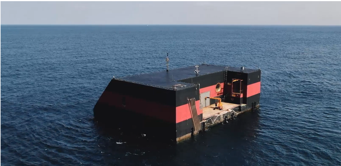
Figure 1: 500kW OWC-WEC at Yongsoo, Jeju, South Korea.
