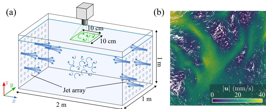
Figure 3: (a) A schematic of the turbulent water tank and camera arrangement. The green shaded area represents the FOV. (b) A snapshot of particle trajectories on the free surface in the FOV at  $Re_\lambda = 312$ . The trajectories are color coded by the velocity magnitude.
