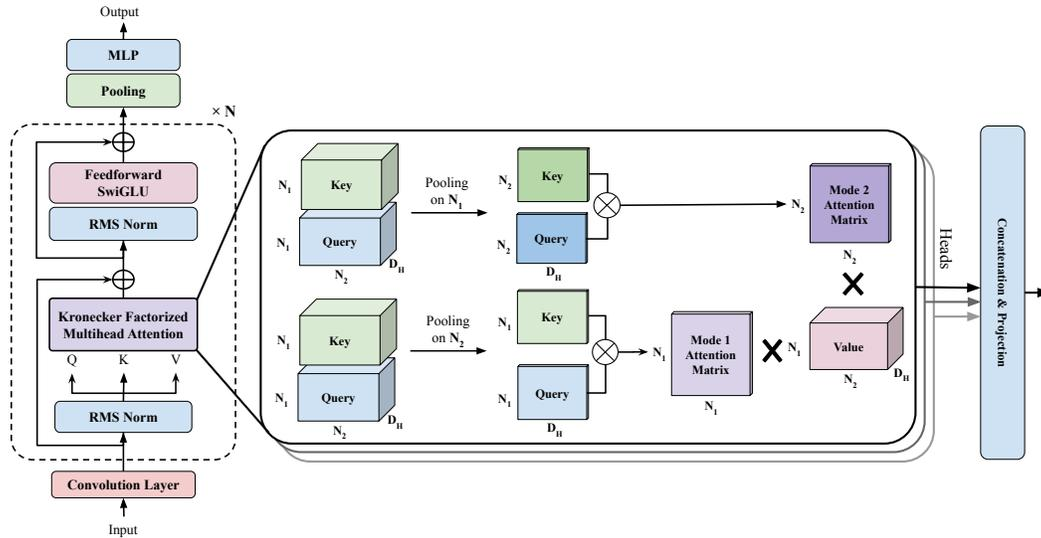
Figure 1: Overall structure of High Order Transformer (HOT) depicting the proposed method for 2D data with size  $N_1 \times N_2 \times D$ . The model shares the same arrangement with the Transformer encoder while employing Kronecker Factorized Multihead Attention, to reduce the computational complexity. Each mode of the tensor (e.g.,  $N_1, N_2$ ) has its own attention matrix, and these are combined using the Kronecker product.
