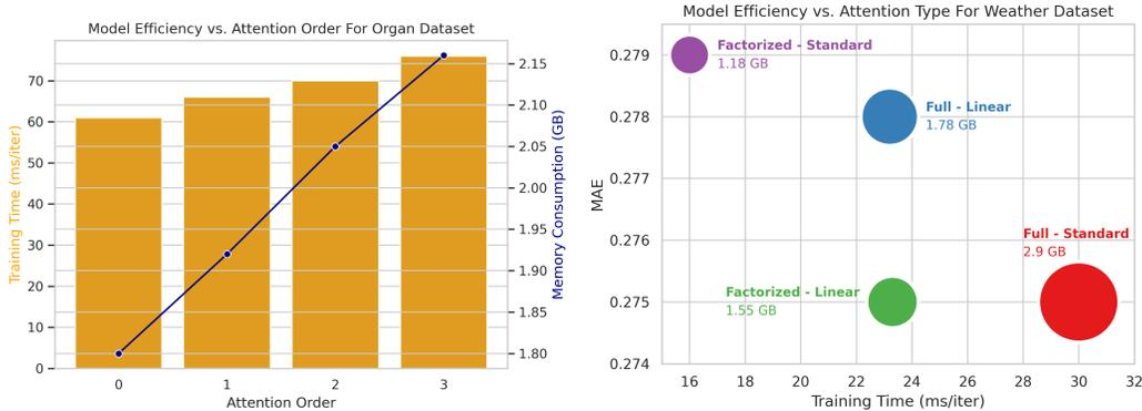
Figure 4: **Left:** Memory footprint and training time of HOT under various attention orders. **Right:** Performance vs. training time of HOT under various attention types. The size of each circle indicates its relative memory consumption. Note that the number of model parameters is fixed for each dataset.
