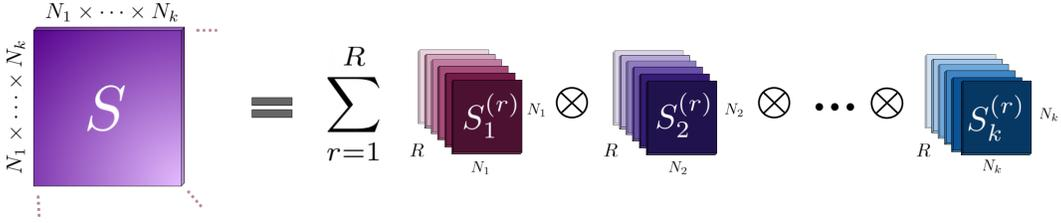
Figure 2: Visualization of a rank  $R$  Kronecker Decomposition of a high-order full attention matrix  $S \in \mathbb{R}^{N_1 N_2 \dots N_k \times N_1 N_2 \dots N_k}$  with factor matrices  $S_i \in \mathbb{R}^{N_i \times N_i}$ . Note that the actual full attention matrix on the LHS can be potentially much larger than what is depicted in the figure.
