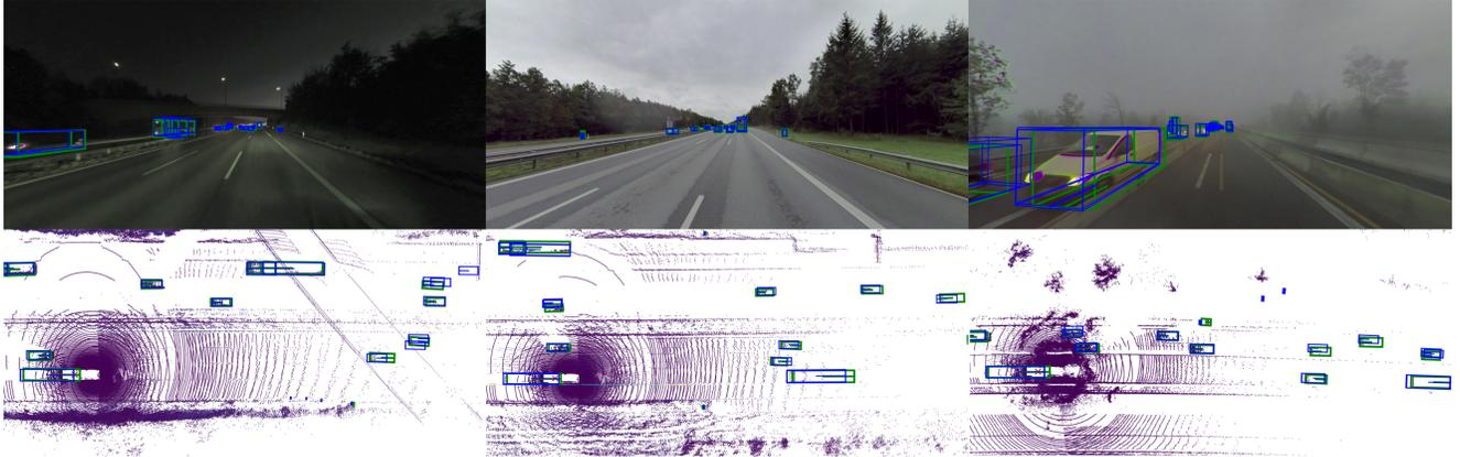
Figure 4. **Qualitative Results** of SpaRC performing in challenging conditions (night, long distance, fog) of the TruckScenes validation set. We visualize the front camera and the corresponding top-down view of the driving corridor with up to 150 m of detection range. Predictions are visualized with blue bounding boxes and annotations in green. LiDAR is displayed for geometric context.
