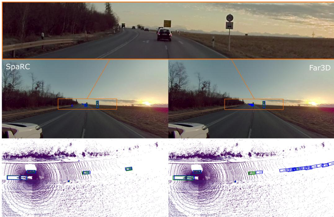
Figure 10. **Qualitative Comparison of SpaRC and Far3D: Sunset Drive.** We visualize predictions (blue) vs ground truth (green) of 3D object detection on the TruckScenes val set in the perspective and top-down view (150 m detection range). SpaRC is visualized on the left and Far3D on the right. The top row shows a zoomed-in cutout of the long-range detection region for better visibility.
