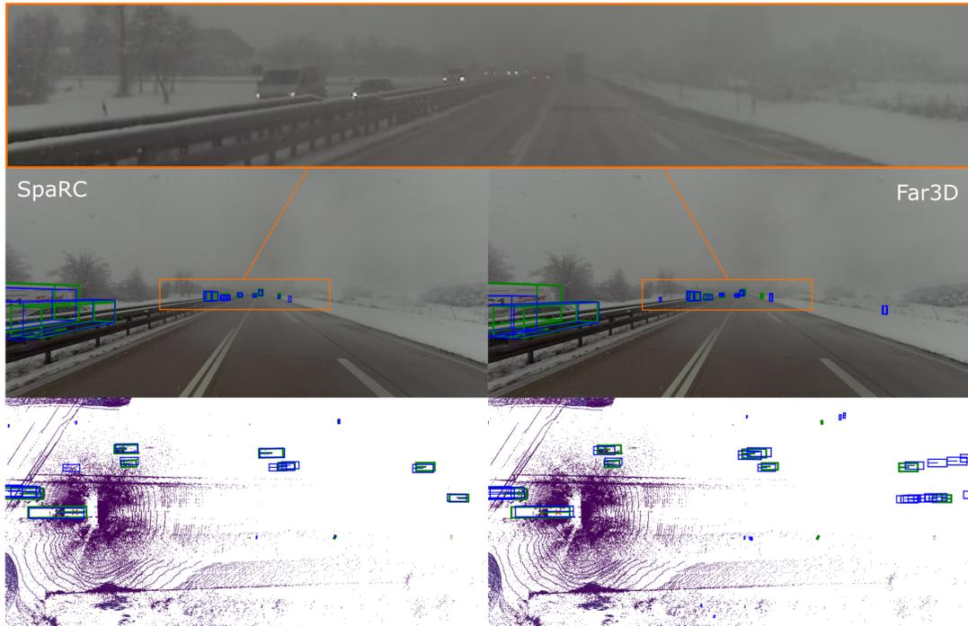
Figure 11. **Qualitative Comparison of SpaRC and Far3D: Winter Scenario.** We visualize predictions (blue) vs ground truth (green) of 3D object detection on the TruckScenes val set in the perspective and top-down view (150 m detection range). SpaRC is visualized on the left and Far3D on the right. The top row shows a zoomed-in cutout of the long-range detection region for better visibility.
