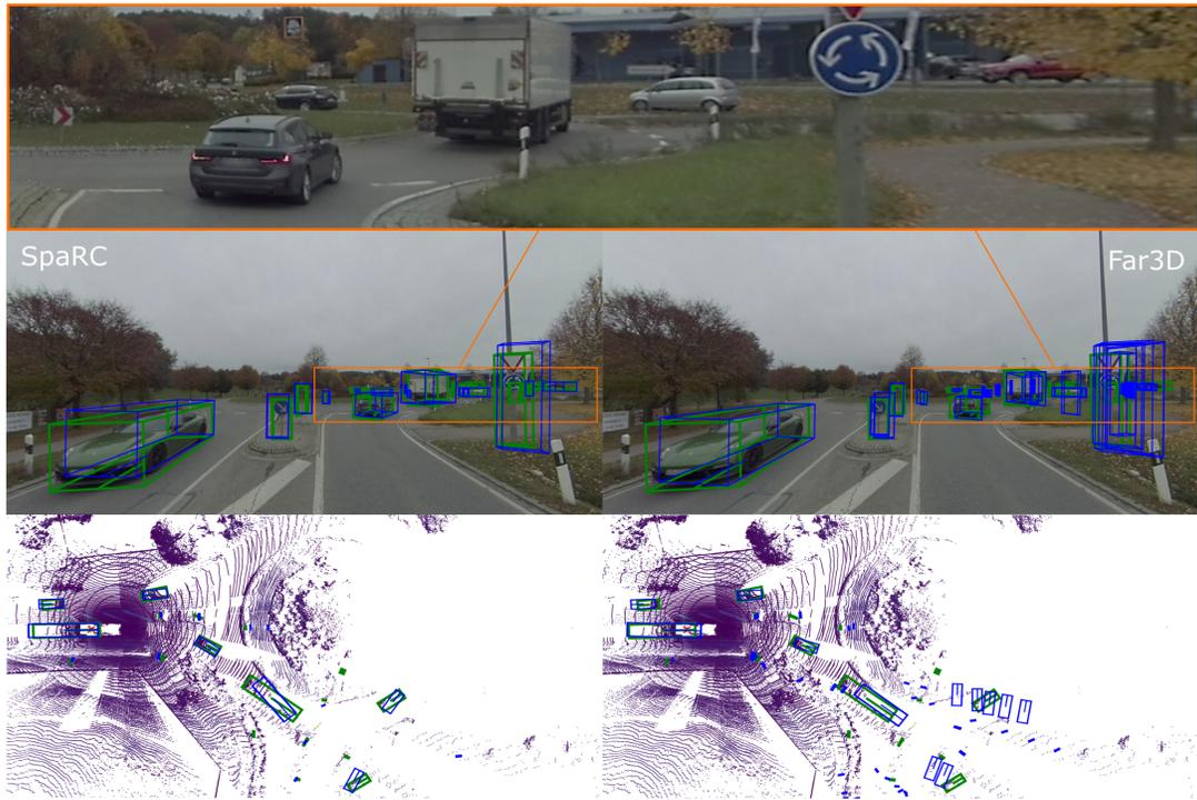
Figure 9. **Qualitative Comparison of SpaRC and Far3D: Roundabout Traffic.** We visualize predictions (blue) vs ground truth (green) of 3D object detection on the TruckScenes val set in the perspective and top-down view (150 m detection range). SpaRC is visualized on the left and Far3D on the right. The top row shows a zoomed-in cutout of the long-range detection region for better visibility.
