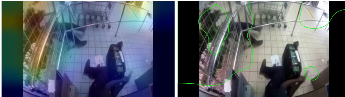
Figure 4.4: Activation map and contour visualization on an image from the gunshot class
