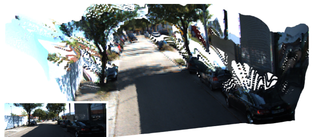
Figure 3. Rendered 3D point cloud from MonoPP on a KITTI Eigen split test sample (unseen during training). Input image is shown at the bottom left.
