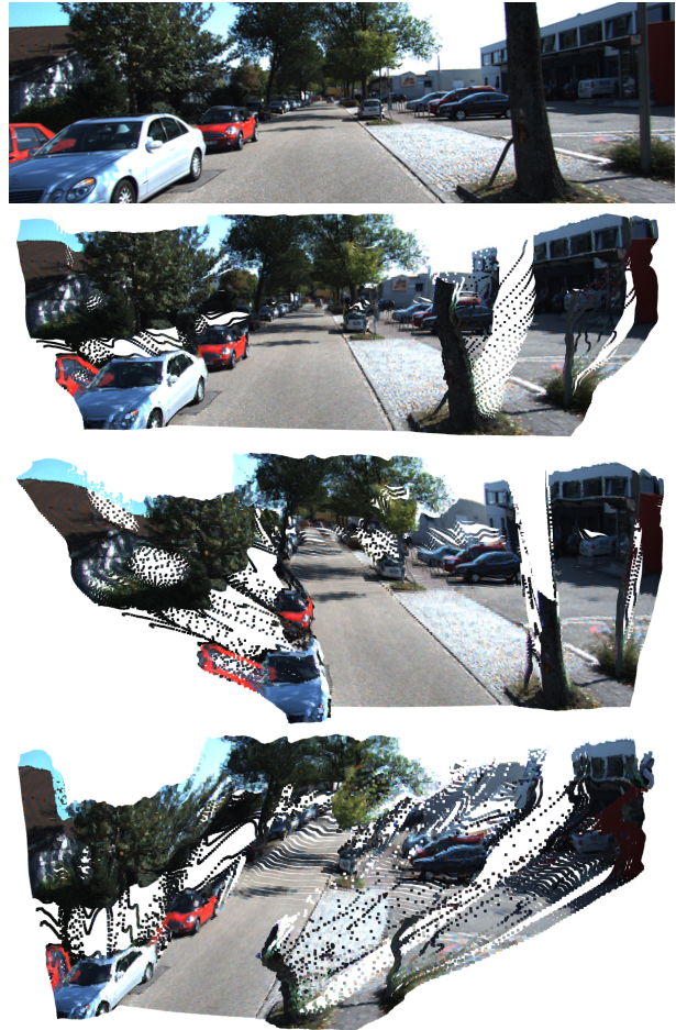
Figure 14. Rendered a 3D point cloud for KITTI data using MonoPP, based solely on a single 2D image input. Multiple view angles were used to visualize the scene.
