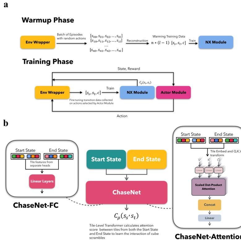
Figure 2.2. The NX Module a. The NX Module training process is divided into a warmup phase and a training phase. b. Two architectural variants of ChaseNet: ChaseNet-FC (fully connected) and ChaseNet-Attention (attention-based).
