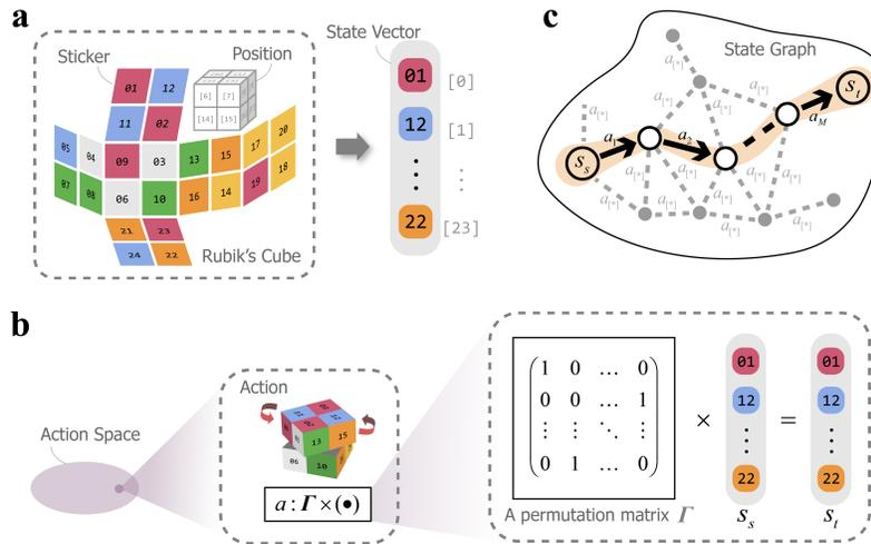
Figure 2.1. General Representation of Rubik’s cube problem. a. The state of the cube can be represented by a vector, with each sticker encoded as a number. b. Scrambles are modeled using a permutation matrix applied to the state vector. c. The cube’s topological structure is visualized as a state graph, where nodes represent states and edges represent transitions.
