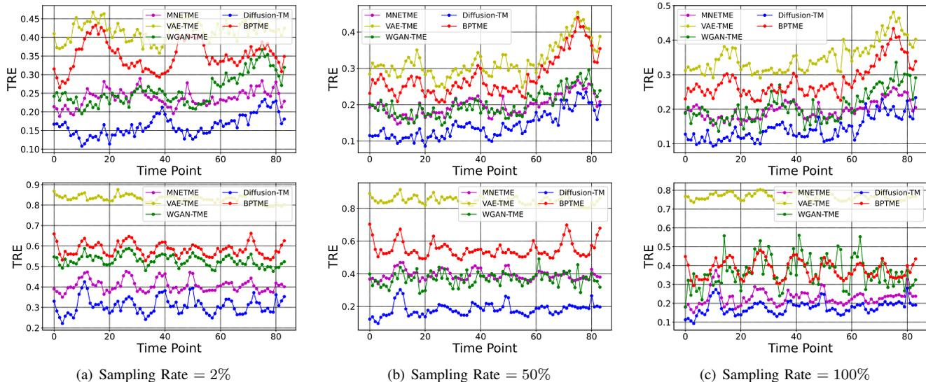
Fig. 9. Temporal relative errors (TREs) on three sampling rates in Abilene (top) and GÉANT (bottom) dataset. For better visualization, the 672 instances were aggregated into 84 records in both datasets.
