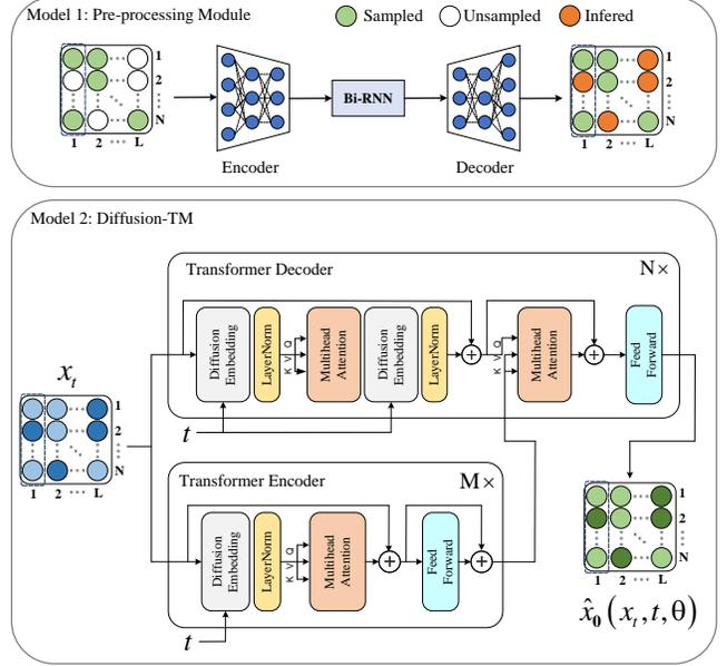
Fig. 5. **(Top) Architecture of Pre-processing Module.** The training of diffusion models starts with a AutoEncoder-based pre-processing module, which generates coarse-grained estimations of missing values in training set. **(Bottom) Overall model structure of Diffusion-TM.** The underlying Transformer is fed a TM sequence  $x_t$  in a diffusion step  $t$ , as well as  $t$  itself, then the diffusion model predicts the clean sample  $\hat{x}_0$ .
