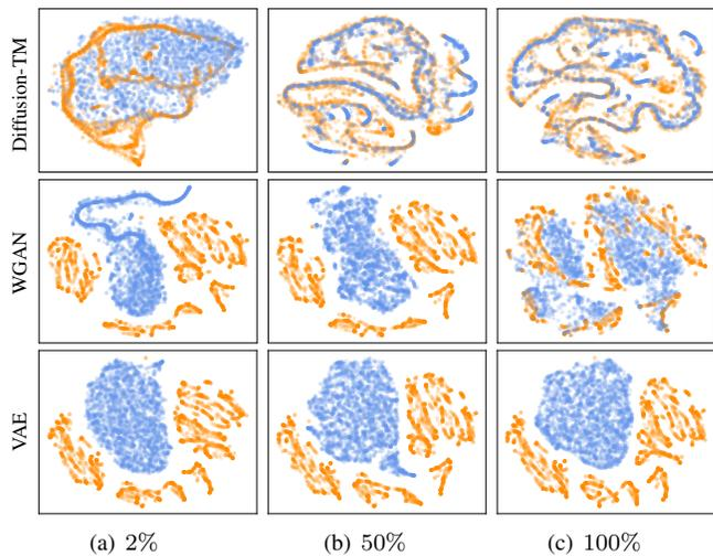
Fig. 7. t-SNE plots for Diffusion-TM (1st row), WGAN (2nd row), VAE (3rd row) in GÉANT dataset with different sampling rates (2%, 50%, 100%) of training traffic traces.
