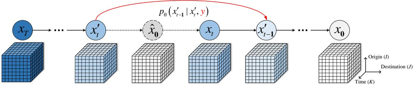
Fig. 3. **Illustration of our diffusion-based approach for solving TM estimation problems.** The reverse inference process (from right to left) iteratively denoises the target traffic matrix  $\mathbf{x}_0$  conditioned on the measurement  $\mathbf{y}$ . Concretely, following the prediction of the estimated  $\hat{\mathbf{x}}_0$  by an unconditional diffusion model, the measurement  $\mathbf{y}$  is incorporated by solving a proximal subproblem depicted by red arrows in the VP-SDE.
