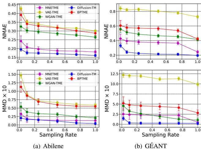
Fig. 8. Network tomography performance for complete TM estimation under different sampling rates.
