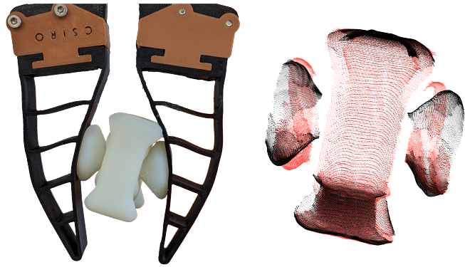
Fig. 1. The SoGraB method: (Left) A soft, Shore 40A object grasped by a soft Fin-Ray gripper. (Right) The extracted point clouds showing initial state (black) and deformed state during grasping (red). By comparing the two states as well as the grasp success, we produce a grasp quality benchmark.
