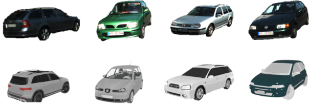
Figure 7. Pose matching results. It shows that the pose of retrieved CAD models (second row) can match accurately with the pose of the input vehicle images (first row) despite the large difference between appearance and geometry.
