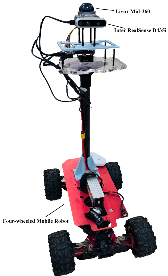
Fig. 10: Four-wheeled mobile robots equipped with sensors employed for conducting experiments in real-world environments.
