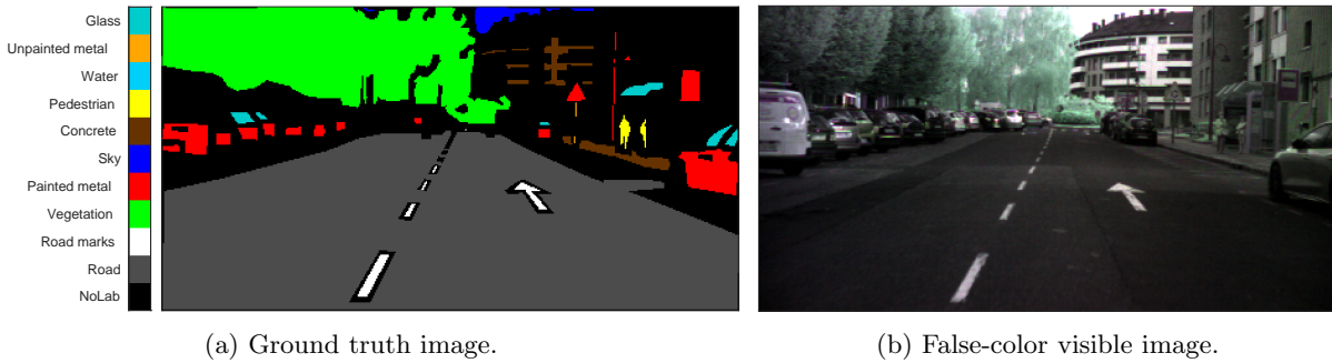
Fig. 1: Ground truth image (a) and its corresponding false-color visible image (b) of an urban scenario as an example of the weak labelling methodology followed to develop the HSI-Drive dataset.
