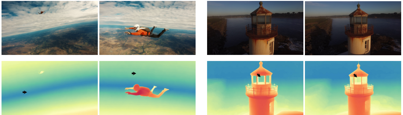
Figure S3. The two samples on the left show incorrect depth predictions in the cloudy sky. The two samples on the right show inconsistencies between different frames of the same video, where the depth at the glass windows fluctuates between the solid and transparent states.
