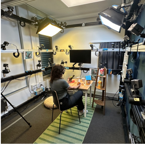
Figure 5. Motion-capture lab. The HOT3D dataset was collected using a motion-capture rig equipped with a few dozens of infrared exocentric OptiTrack cameras and light diffuser panels for illumination variability.
