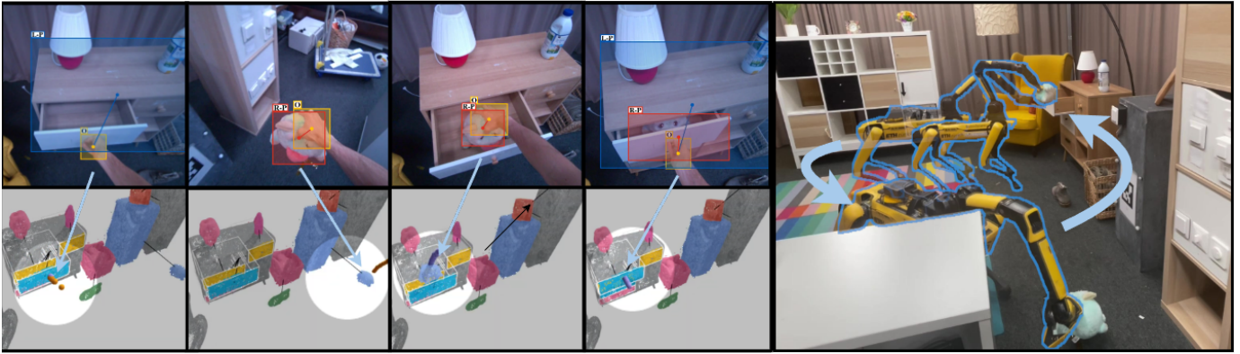
Fig. 3. Teach & Repeat Experiment. We showcase how Lost & Found can help to record reoccurring motion primitives. In this example (from left to right), a human agent opens the top-left drawer of the small cabinet and grabs the blue toy from the other side of the room. The toy is then stored inside the drawer. To conclude the action, the drawer is closed again. We demonstrate that our method can be seamlessly integrated into robotic systems that are then capable of replaying the tracked interaction (on the right).
