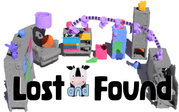
Fig. 1. Object tracking : Our method allows to track the dynamic information associated with the pick-and-place action of the cow toy (purple). The figure presents a series of snapshots of the employed scene graph data structure at varying time points. The object trajectory extends from the right shelf to the top-left drawer of the cabinet, as indicated by the dotted arrow.
