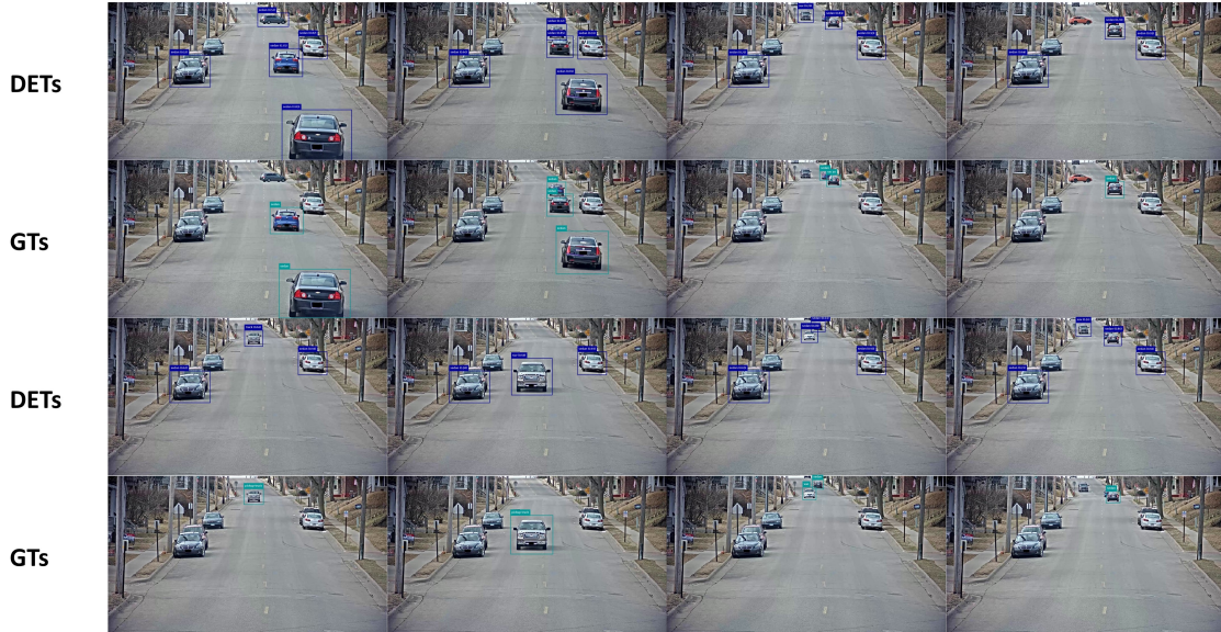
Figure 2: Qualitative Analysis of the proposed Co-Learning solution on the 7th AI CITY CHALLENGE Track 2 dataset. The base detector is Faster-RCNN with ResNet-50 as the feature extractor for all experiments to ensure a fair comparison. ( DETs: Detected Results, GTs: Ground Truths )
