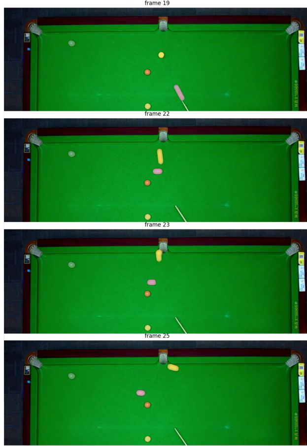
Figure 13: Segmentation mask rendering of the Det-SAM2-pipeline in our self-implemented billiard scene example. The Det-SAM2 framework is able to maintain the original segmentation capabilities of SAM2 while operating autonomously.
