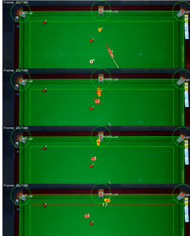
Figure 12: The visualized post-processing result of the Det-SAM2-pipeline in our self-implemented billiard scene example is shown in Figure 13. This image was derived from the segmentation masks predicted by SAM2, followed by post-processing. As seen, with the support of SAM2, even though the fast-moving balls are stretched in the camera frame, they are still perfectly captured.
