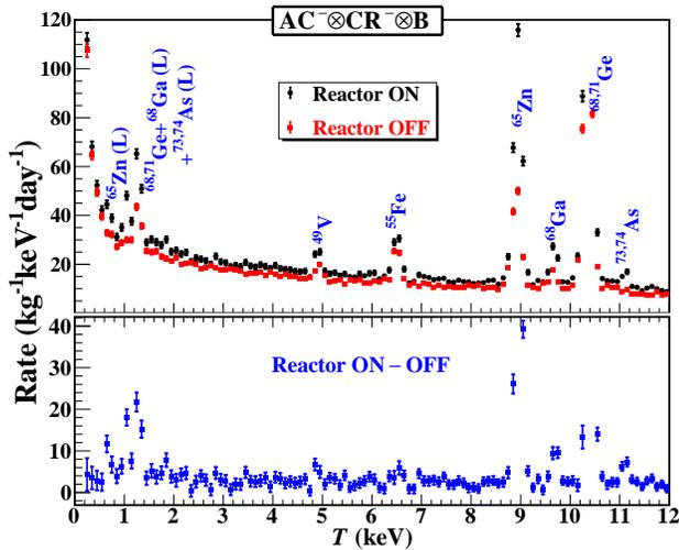
FIG. 3. (Top) Candidate  $\nu A_{eI}$  spectra from 242(357) kg-days of Reactor ON(OFF) data. The cosmogenic X-ray lines are identified. (Bottom) Reactor ON–OFF spectrum showing the finite  $^{135}\text{Xe}$  Compton excess. Cosmogenic peaks are observed for those isotopes with half-lives comparable to the data taking duration. The 10.37 keV X-ray peak extends off-scale and is truncated for clarity in display.
