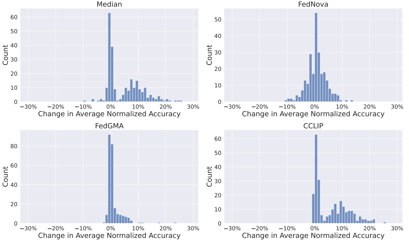
Figure 1: Histograms showing the change in average normalized accuracy for four different methods compared to Task Arithmetic. For each plot, the x-axis represents the change in average normalized accuracy, calculated as the difference between the average normalized accuracy of the algorithm used and that of Task Arithmetic. The y-axis indicates the number of experiments within the range of change values. A positive value on the x-axis indicates that the algorithm improves upon Task Arithmetic, while a negative value indicates that the algorithm degrades Task Arithmetic.
