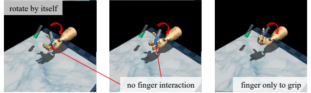
Figure 2. Demonstration of ghost states on the pen reorientation task. The visualizations are rendered by setting predicted states frame by frame, which cannot actually happen and will lead to failure. The pen appears to autonomously rotate to the desired pose without any hand manipulation, and the fingers look like moving to grasp the pen at the last frame.
