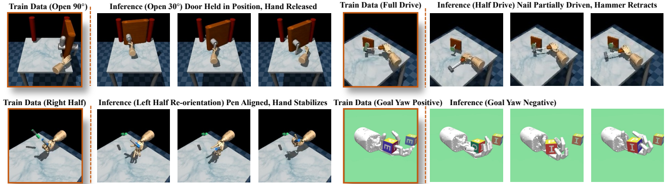
Figure 4. Visualization results of goal-adaptive tasks by DexHandDiff. For each task, training data sample (with orange stroke) is followed by inference on novel goals beyond the training data. In the Door task, DexHandDiff guides the door to new target angle (30°) and holds the door in position when the hand releases, which cannot be attained by simply truncating actions from 90° training data. DexHandDiff avoids ghost states and achieves better goal adaptability.
