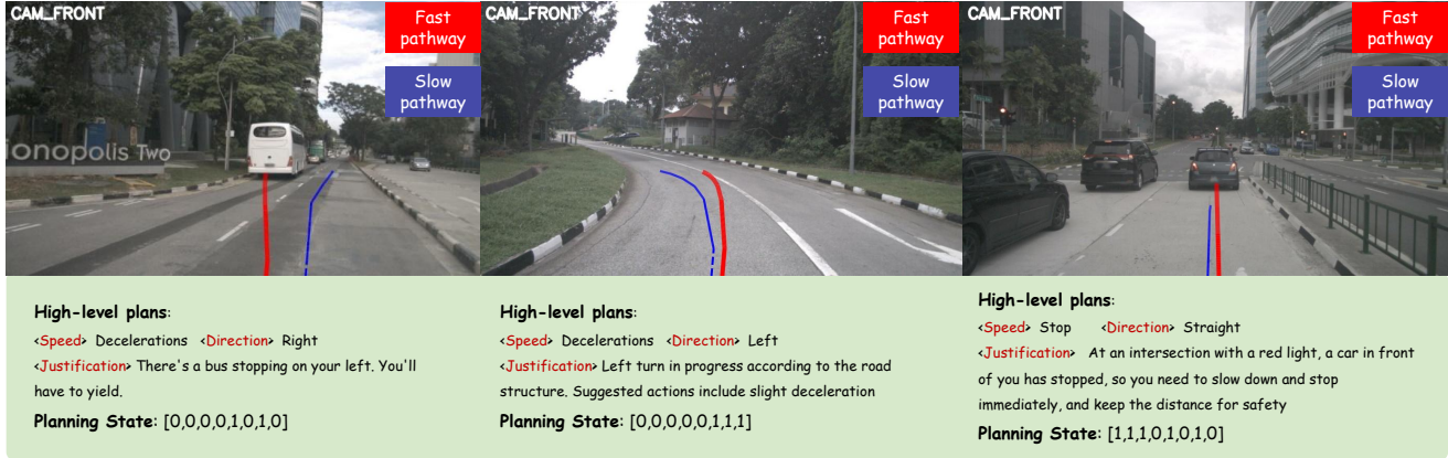
Figure 4. Example scenarios demonstrating FASIONAD’s adaptive feedback framework in various driving environments. Each scene shows different navigation challenges, including obstacles, lane adjustments, and turns. The proposed system provides suggested driving operations and ensures safe, smooth trajectories with minimal abrupt maneuvers, enhancing navigation performance and safety in complex situations.
