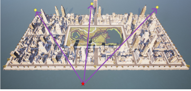
Fig. 3: Training flight paths. The yellow six-pointed stars represent the targets, the red star indicates the fixed-wing UAV’s take-off position, and the purple line represents the expected flight trajectory.
