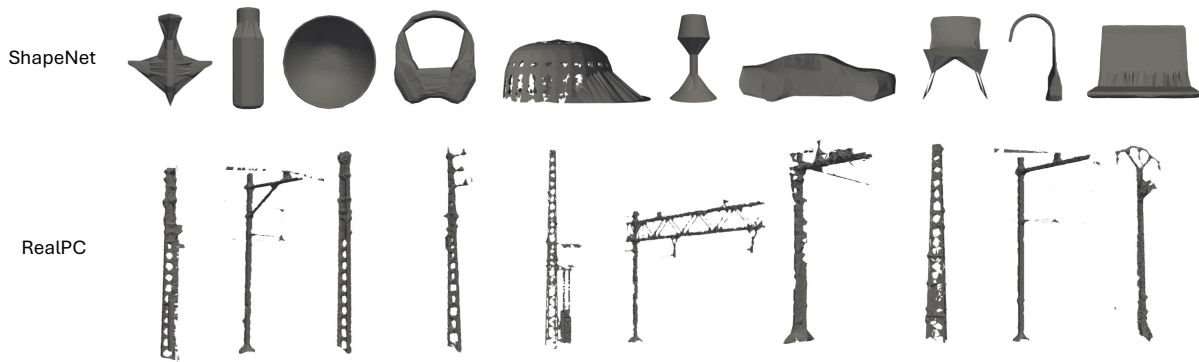
Figure 12: Surface reconstruction of some instances from different categories of ShapeNet and RealPC using alpha shapes.
