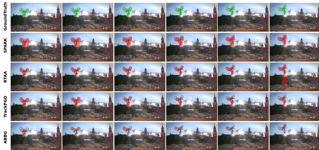
Figure 5: Several examples of TransT-M (Chen et al., 2023) performance after applying the white-box attacks containing SPARK (Guo et al., 2020) (blue), RTAA (Jia et al., 2020) (black), TrackPGD (Nokabadi et al., 2024) (white), and our proposed ABBG attack (red) binary masks. The Green color represents the ground truth (mask).
