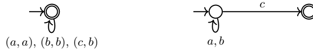
Fig. 3. Left: A transducer \mathcal{T} that converts each occurrence of letter c into letter b . Right: A weakly acyclic DFA \mathcal{A} accepting language (a + b)^*c .
