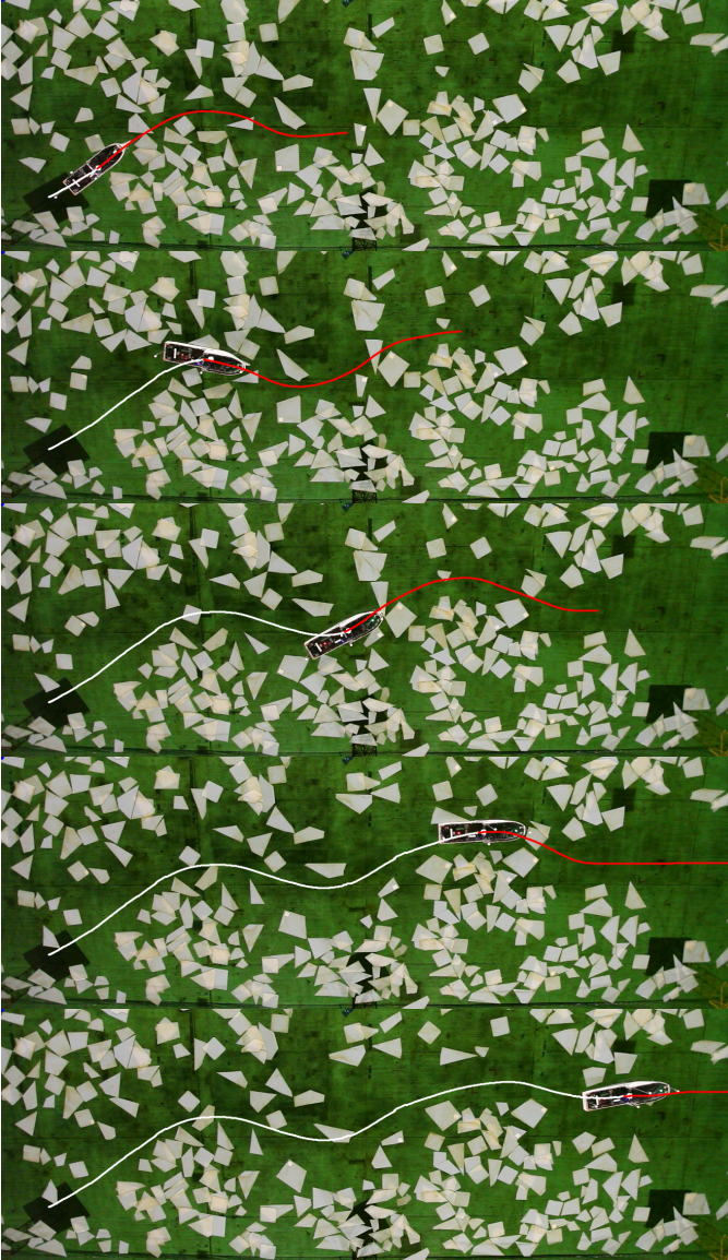
Fig. 17: Five snapshots from a sample AUTO-IceNav trial, displaying the planned path in red and the actual ship path in white. Videos of trials can be found at https://github.com/rdesc/AUTO-IceNav#demo-videos-from-nrc-experiments .
