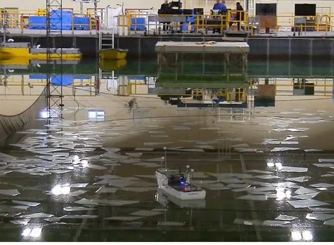
Fig. 14: Side view of the experimental setup in the Offshore Engineering Basin research facility. The ice basin contains a collection of plastic ice pieces cut from sheets of polypropylene.
