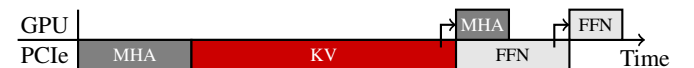
(a) Naive offloading pipeline for row-by-row schedule with asynchronous data transfer. GPU and PCIe denote GPU computation and data transfers, with arrows indicating data dependencies.
