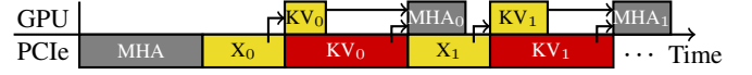
Figure 4: Offloading pipeline for column-by-column schedule with partial KV cache recomputation to maximize throughput.
