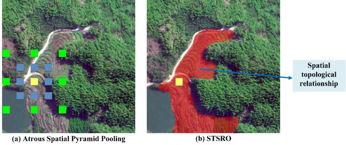
Fig. 5. Illustrating the STSRO spatial topological semantic relationship for the pixel marked with the yellow square. (a) Atrous spatial pyramid pooling: the multi-scale context is a set of sparsely sampled pixels marked with blue squares and green squares. The pixels exhibiting different colors are indicative of disparate dilation rates. These pixels are dispersed throughout both the object region and the background region. (b) STSRO: The spatial topological semantic relationship is expected to be a set of pixels lying in the object (marked with color red).
