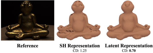
Figure 9. We demonstrate the differences between SH and latent color representations on the “scan110” sample of the DTU dataset. When reconstructing specular surfaces (left), the SH representation (middle) leads to visible holes in the recovered mesh; these artifacts are resolved when using a latent representation (right).
