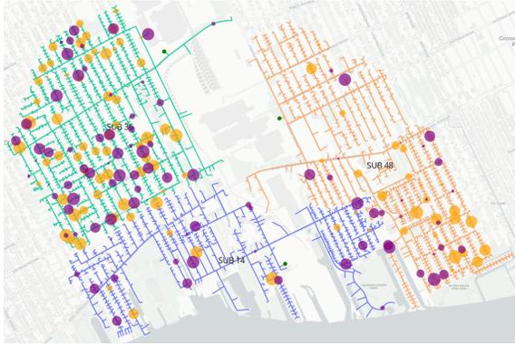
Fig. 7. Optimal sizes and locations of solar panels and batteries in three substation service areas (*SUB14*, *SUB36*, and *SUB48*). Purple dots represent batteries, and yellow dots represent solar panels. The size of the dot is proportionate to the installed capacity.
