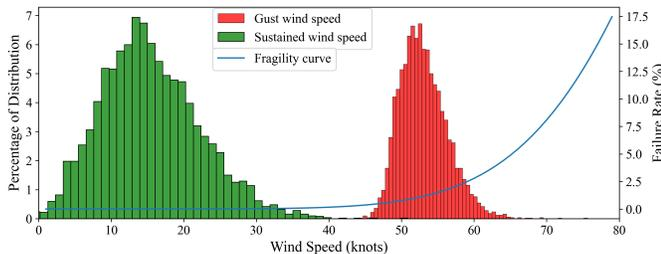
Fig. 2. Wind speed distribution of gusts and sustained winds, along with the wind speed-based fragility curve.
