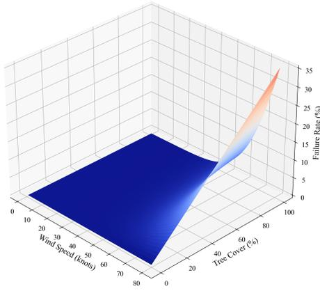
Fig. 4. Fragility curve illustrating the joint influence of wind speed and tree coverage.
