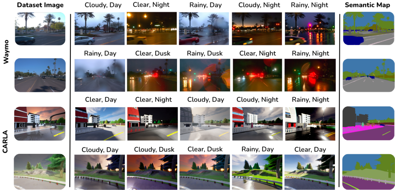
Figure 1. Qualitative visualizations of synthetic images generated by SynDiff-AD across various subgroups for the semantic segmentation (Waymo) and autonomous driving tasks (CARLA). We qualitatively visualize synthetic variants for an image in the original dataset (first column) and its corresponding semantic mask (last column). The original dataset images belong to over-represented data subgroups, such as “Cloudy, Day” and “Clear, Day”, for both the semantic segmentation and autonomous driving tasks. We leverage our data augmentation pipeline, SynDiff-AD , to generate images for different under-represented subgroups (illustrated in columns 2 to 6).
