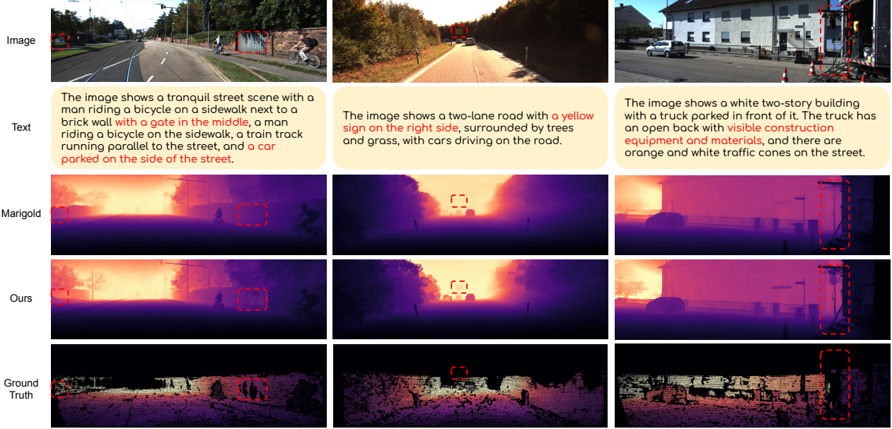
Figure 4. Visualization on KITTI. Compared to Margold, our PriorDiffusion model shows superior accuracy in depth prediction for a given input image, especially for objects highlighted in the language description (marked in red), even when parts of the object are almost visible in the image (such as the parking car in the first column). This shows that the language prior can help the model better infer the geometric properties of these objects and improve distance estimation. Furthermore, the language descriptions guide the model’s attention to specific regions relevant to user needs, such as a sign at a distance, which can potentially enhance the safety of self-driving systems that rely solely on vision sensors.
