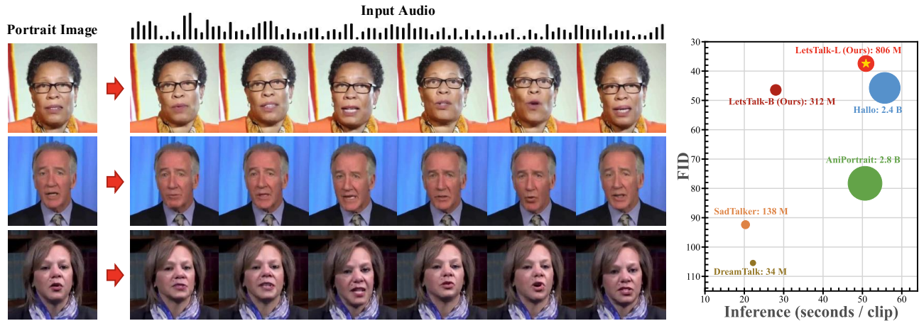
Figure 1. We propose LetsTalk , a diffusion-based transformer for audio-driven portrait image animation. Left : Given a single reference image and audio, LetsTalks can produce a realistic and vivid video aligned with the input audio. Note that each column corresponds to the same audio. The results show that LetsTalk can drive consistent and reasonable mouth motions for the input audio. Right : Generation quality vs. inference time on the HDTF dataset, the circle area reflects the number of parameters of the method. Our LetsTalk achieves the best quality while also being highly efficient in inference, compared to current mainstream diffusion-based methods such as Hallo and AniPortrait. In addition, our base version ( LetsTalk-B ) achieves performance similar to Hallo with only 8 \times fewer parameters.
