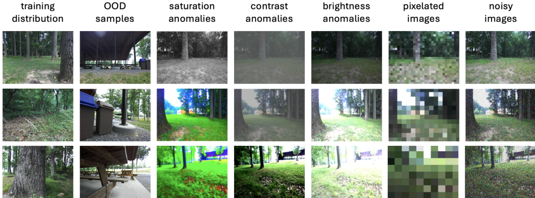
Figure 3. Example images from the outdoor park dataset. Column 1: test images drawn from the same distribution as the training images (forested/grassy regions). Column 2: test images associated with unexplored regions drawn from a new distribution (regions around pavilion). Column 3: test images with varied saturation levels generated from in-distribution images. Column 4: test images with varied contrast levels generated from in-distribution images. Column 5: test images with varied brightness levels generated from in-distribution images. Column 6: in-distribution images that have been pixelated. Column 7: in-distribution images with additive noise.
