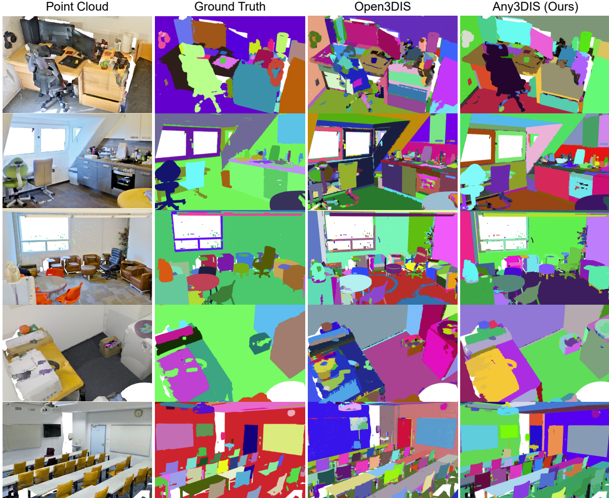
Figure 4. Qualitative Result on ScanNet++ Validation Set. : From left to right we show the input point cloud of 3D scenes, GT segmentation, Open3DIS [19], and Any3DIS (ours) results. Our approach achieves more accurate and consistent segmentation than Open3DIS.
