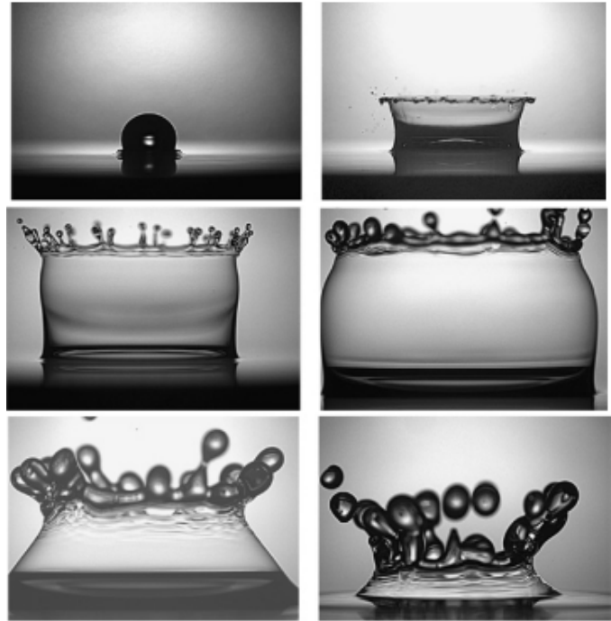
Fig. 2: Droplet impact captured using high-speed photography techniques [9]
