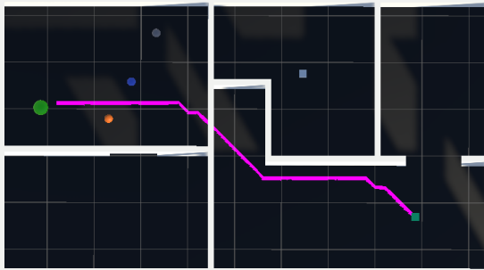
FIGURE 7. Naive A* Pathfinding. (Yellow: Chair, Blue: Robot, Gray: Grinder)
