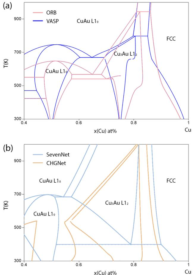
Figure 4: Cu–Au binary phase diagram on the Cu-rich side plotted with (a) VASP and ORB; (b) SevenNet and CHGNet
