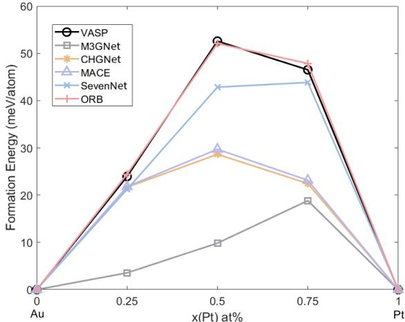
Figure 2: The formation energies of FCC Au–Pt SQS calculated with VASP and MLIP data.
