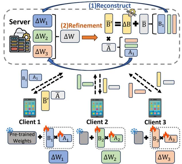
Figure 1. **Illustration of LoRA-FAIR.** Instead of directly averaging the local LoRA modules  $A_k$  and  $B_k$  collected from each client  $k$  on the server side and sending the averaged LoRA modules  $\bar{A}$  and  $\bar{B}$  back to clients, LoRA-FAIR reconstructs the ideal global update  $\Delta W$  using Eq. (7), finds the residual LoRA module  $\Delta B$  using Eq. (8), and replaces  $\bar{B}$  with the corrected LoRA modules  $B' = \bar{B} + \Delta B$ . See details in Sec. 4.
