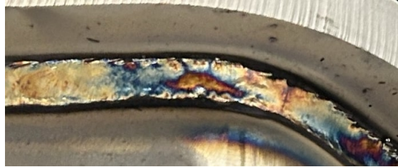
Figure 11: A corner of the workpiece showing significantly improved welding quality after system re-calibration.
