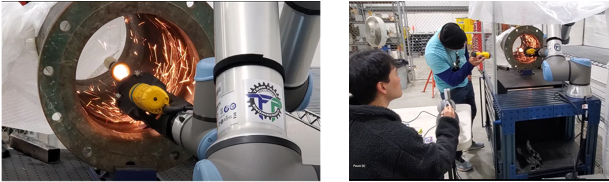
Figure 14. Test Teleoperation of Downhole Weld Bead Removal.
