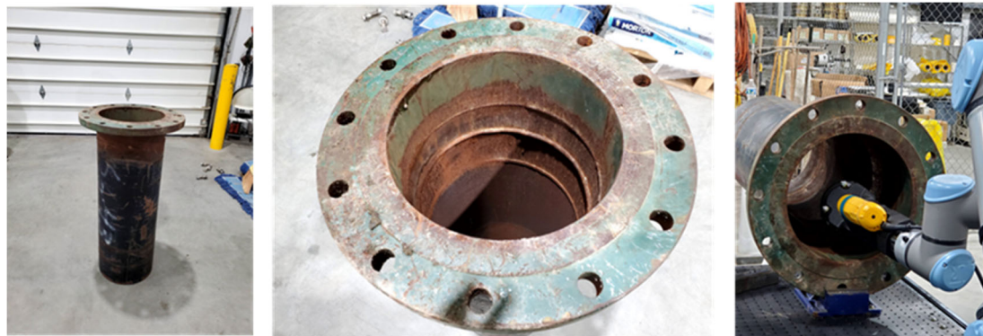
Figure 13. Demonstration Test Object with Downhole Weld Beads.
