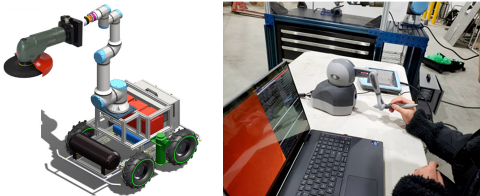
Figure 2. Robotic system with plug-and-play interchangeable tools is being developed by Florida International University
