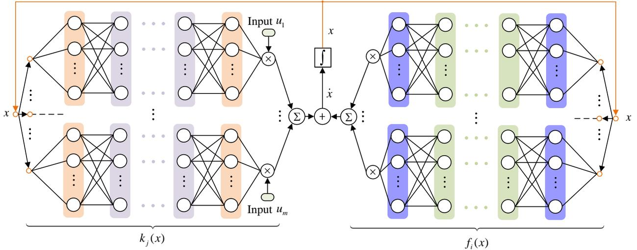
Fig. 1: The schematic of ICODEs. Using the ODE integration methods, it illustrates how the state  $x$  evolves through the external input  $u$  and the neural networks (NNs)  $k_1, \dots, k_m$ , and the NN consisting of the subnetworks  $f_1(\cdot), \dots, f_M(\cdot)$ .
