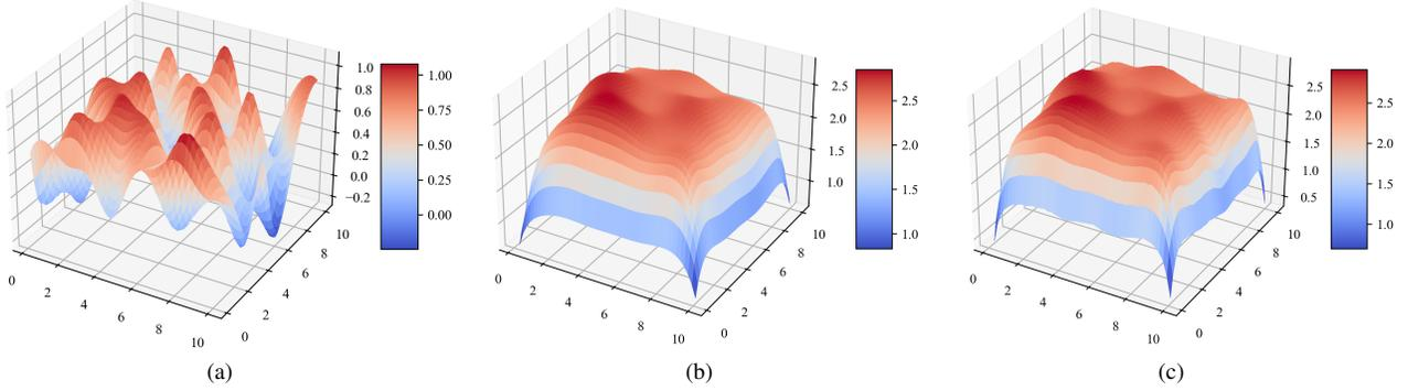
Fig. 10: Displays initial conditions and prediction by ICODE for heat conduction equation, compared with the ground truth. (a) Initial Condition. (b) Ground Truth. (c) Prediction by ICODE.
