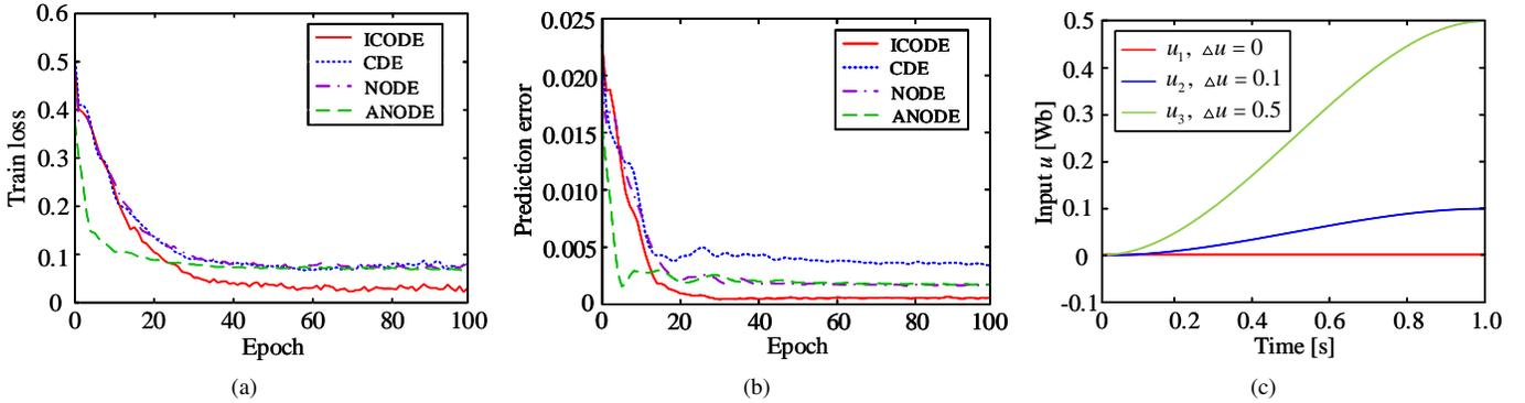
Fig. 2: Comparison of training and prediction errors at each time step on the test set for different models on the task of the single-link robot. (a) Training loss in MSE under  $u_3$ . (b) Prediction loss in MSE under  $u_3$ . (c) Inputs  $u$ .
